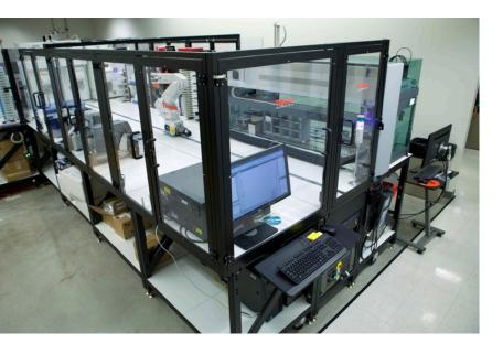
Illinois Biological Foundry for Advanced Biomanufacturing (iBioFAB). iBioFAB is a fully integrated computational and physical infrastructure that supports rapid design, fabrication, validation, and quality control as well as analysis of genetic constructs and organisms. [Courtesy CABBI1
