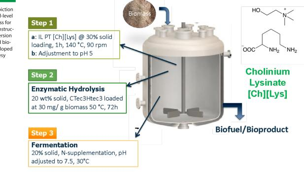
Schematic depiction of an industrial-level one-pot process for biomass deconstruction and conversion to biofuels and bioproducts developed at JBEI. [Courtesy JBEI]
